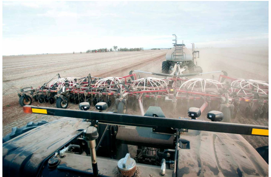
Photo 4: A New Holland T9 tractor with a Case Flexicoil PTX 600 airseeder bar towing a Flexi-Coil 3850 air cart bin used to sow cereal seed.
