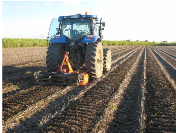
Figure 2: Zonal tillage using a power harrow and crumbler roller was applied to the top of these beds. In this example, different depths of zonal tillage (50 mm and 125 mm) were applied at variable times prior to planting cane in September. The overall objective is to incorporate soybean crop stubble and create a zone conducive to growth of the cane sets whilst retaining the bed structure and controlled traffic zones. (Photos: Alan Munro, Woodford Dale, NSW)
