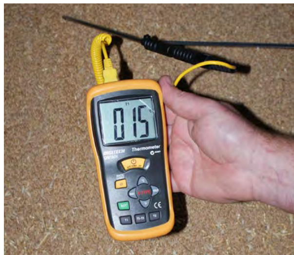
Photo 7: At grain temperatures below 15°C most storage pests stop reproducing. (Source: Chris Warrick, Primary Business)
