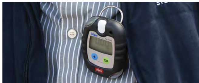
Photo 4: Personal phosphine monitors sound an alarm if harmful concentration levels are detected. (Source: Ben White, Kondinin Group)
