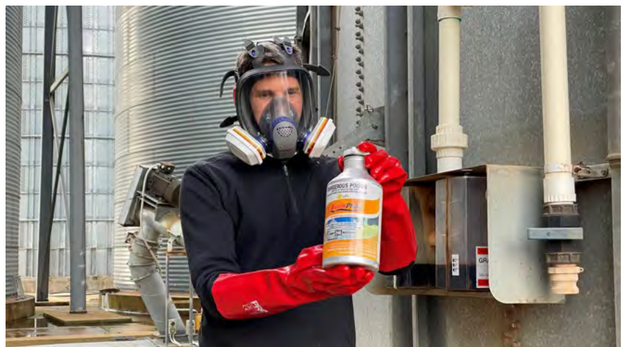
Photo 3: A full-face breathing respirator is required for handling phosphine. The respirator must be fitted with a combined dust and gas cartridge (canister) suitable for inorganic gas. (Source: Ben White, Kondinin Group)
