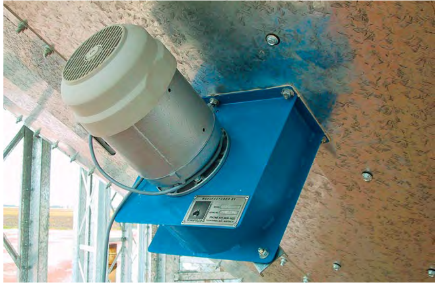
Photo 1: If over-moist grain can't be dried immediately hold it under aeration cooling until drying equipment is available. (Source: Phillip Burrill, DAF QLD)
