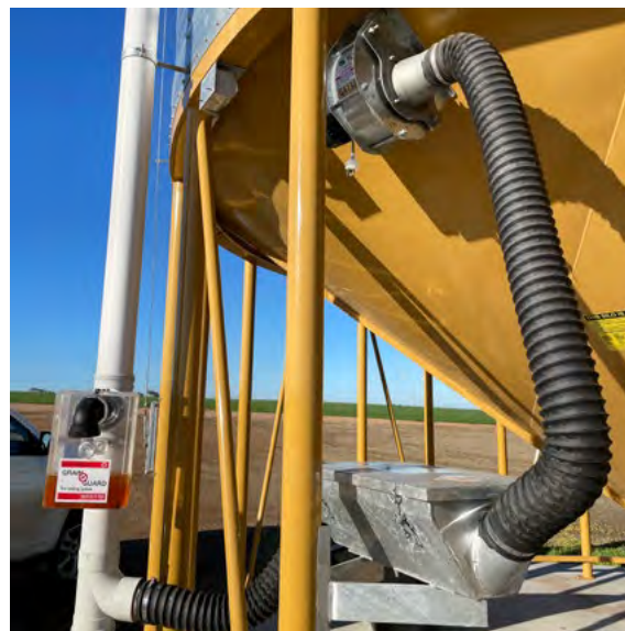
Photo 9: Some silos are built with a chamber and passive (thermo-siphon) or powered recirculation system for applying phosphine from the bottom. (Source: Ben White, Kondinin Group)
