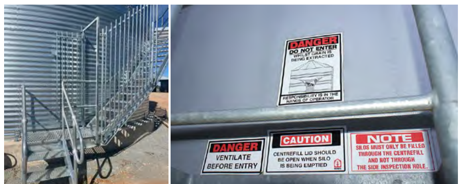
Photo 1: Silos require safe access to the top for monitoring and maintenance. (photo left). (Source: Ben White, Kondinin Group). Place warning stickers on silos near the ladder, where operators will easily see them (photo right). (Source: Chris Warrick, Primary Business)
