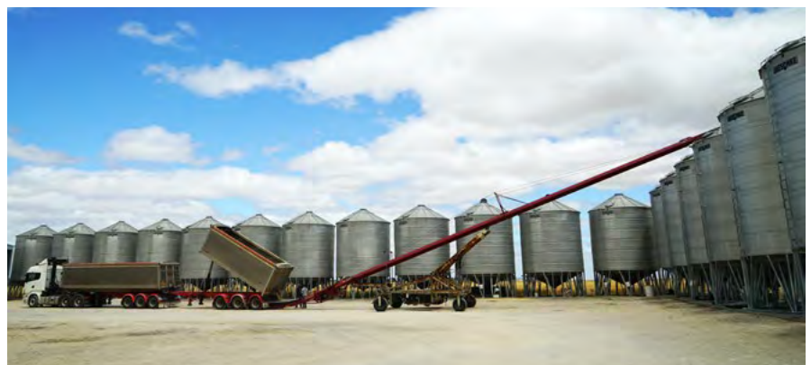
Photo 2: Having a large gravelled area around silos enables machinery to be moved into position safely. Always fill silos from the centre to avoid uneven loading. (Source: Chris Warrick, Primary Business)
