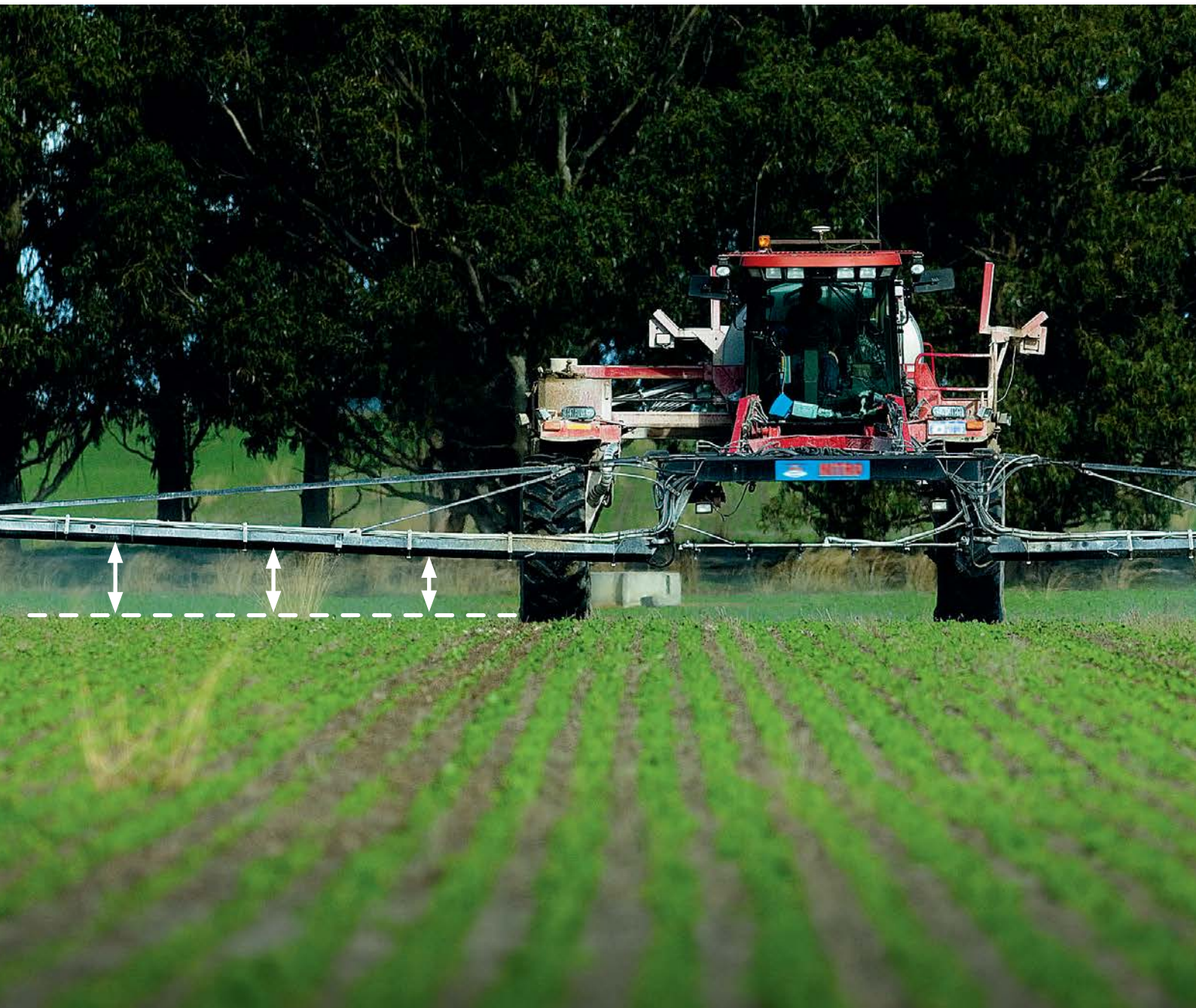
Increasing boom height increases drift risk.
