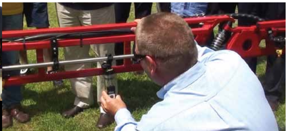
Bill Gordon checking nozzle outputs at an application and drift management workshop in central Queensland.
