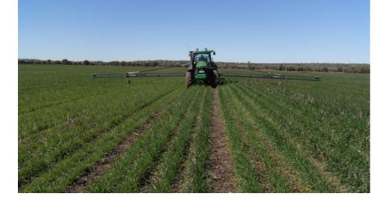
Hayes auto boom height using wheels and a hydraulic load sensor on the ram
