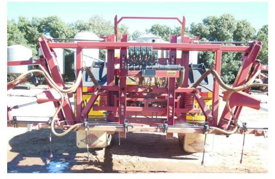
Auto boom height may not work as well unless the boom centre can be made more rigid (for example, with additional boom-roll mechanisms) when the individual boom wings are raised and lowered manually or automatically.
