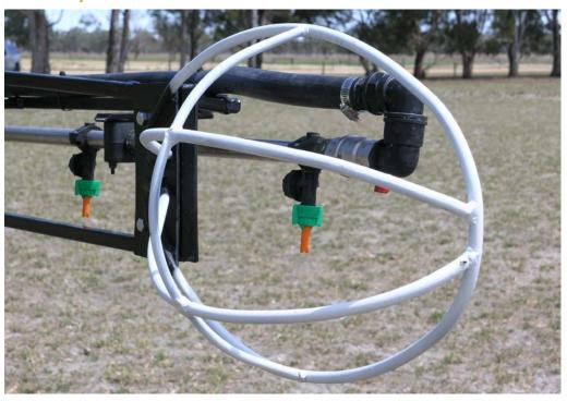
An adapter cap to lower nozzle position
