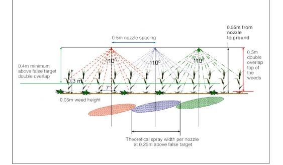
Figure 2 Wrong height above the target leading to uneven application.
