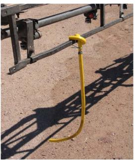
A visual guide on the boom makes it easy to set the correct nozzle height.
