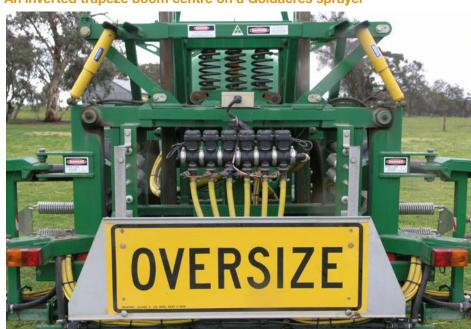
Auto boom height may not work as well unless the boom centre can be made more rigid when the individual boom wings are raised and lowered manually or automatically (for example, boom-roll mechanisms).
