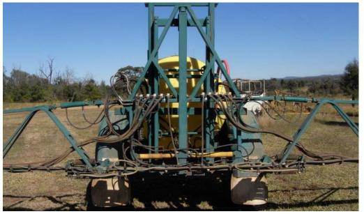
Pendulum boom centres are common on some trailing sprayers and some models of self-propelled sprayers.
