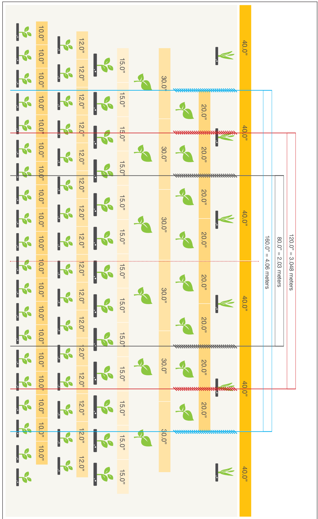
Figure 1 Position of the wheels and traffic in relation to row spacing for an even number of planted rows (based on imperial row spacings).
