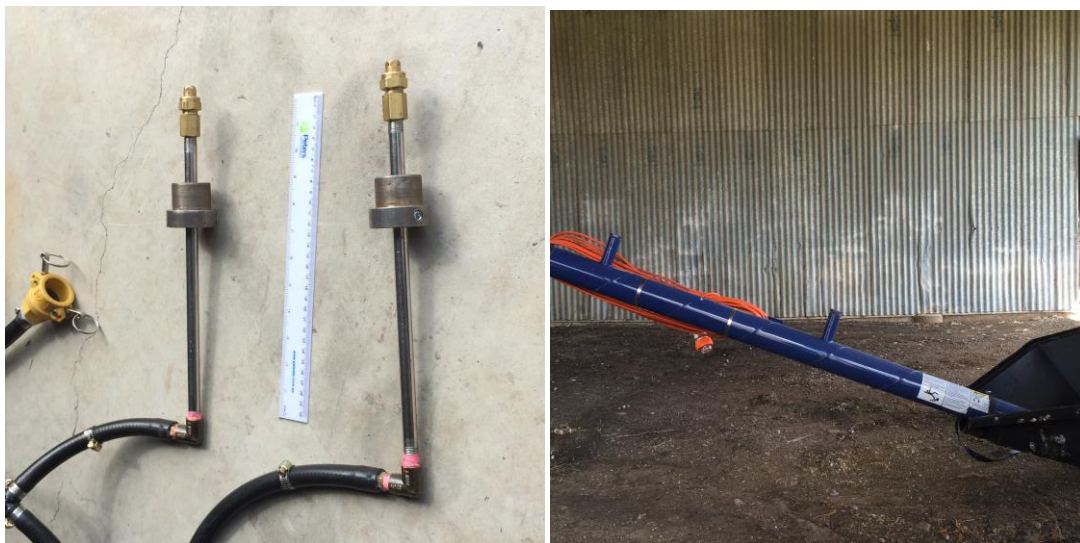
Figure 7. Spray application equipment designed for good coverage by applying treatment at two points in the auger
