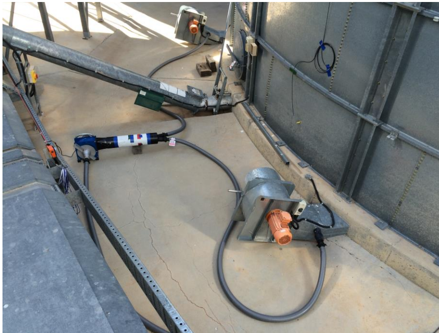
Figure 6. A small fan (F370 – 0.37 kW) used during the first 5 days of fumigation to recirculate phosphine to give rapid uniform gas distribution in 1423 t wheat. See Figure 5.
