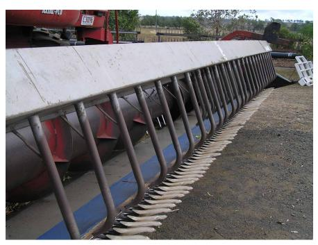
Photo 4: Harvestaire front combined with extension fingers and a blue Vibra-mat. Photo: G. Cumming, Pulse Australia
