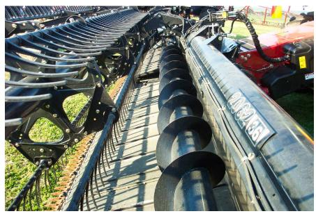
Photo 1: Belt-front fitted with cross-auger. Photo: W. Hawthorne, Pulse Australia
