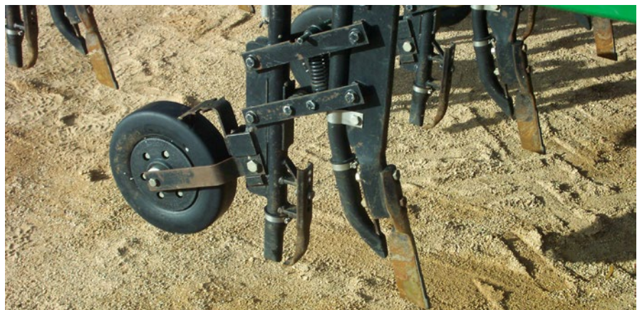
Photo 6: The DBS system parallelogram for uniform seeding depth and deep placement of seed or fertiliser.
