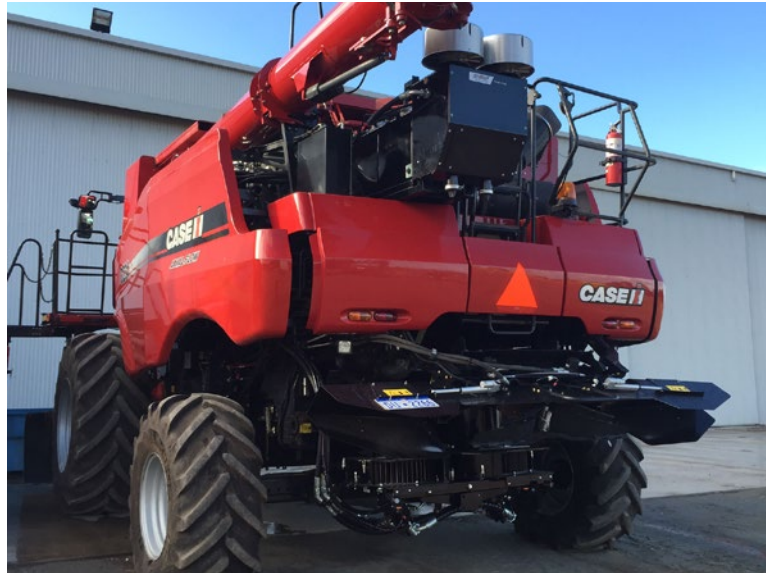
Figure 8: The integrated Harrington Seed Destructor iHSD system is one way to destroy weed seeds at harvest by pulverising the chaff fraction as it leaves the harvester.
