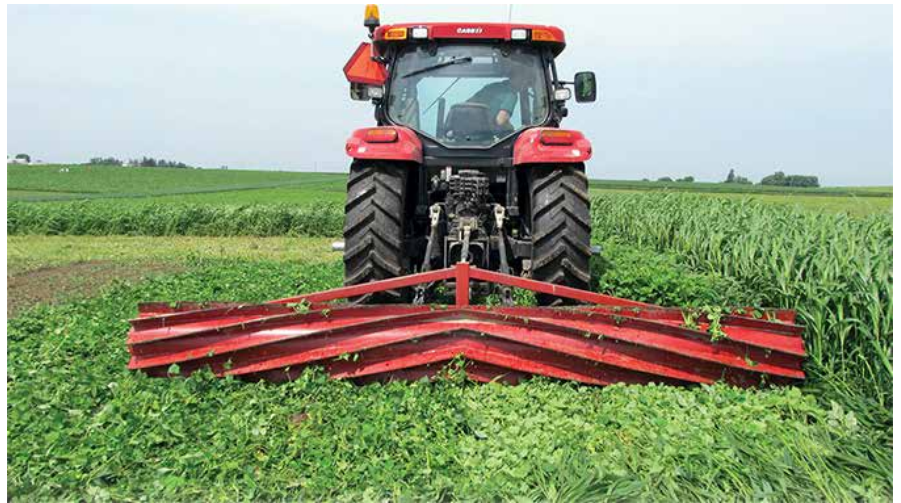
Photo 3: Well-designed roller-crimpers, and a good management plan, can help no-tillers and strip-tillers to smother weeds, improve soil protection and get the most from high-biomass cover crops.
