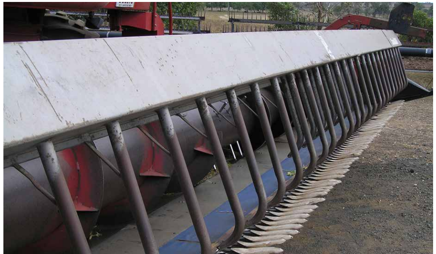
Figure 5: Harvestaire front combined with extension fingers and a blue vibra-mat.
