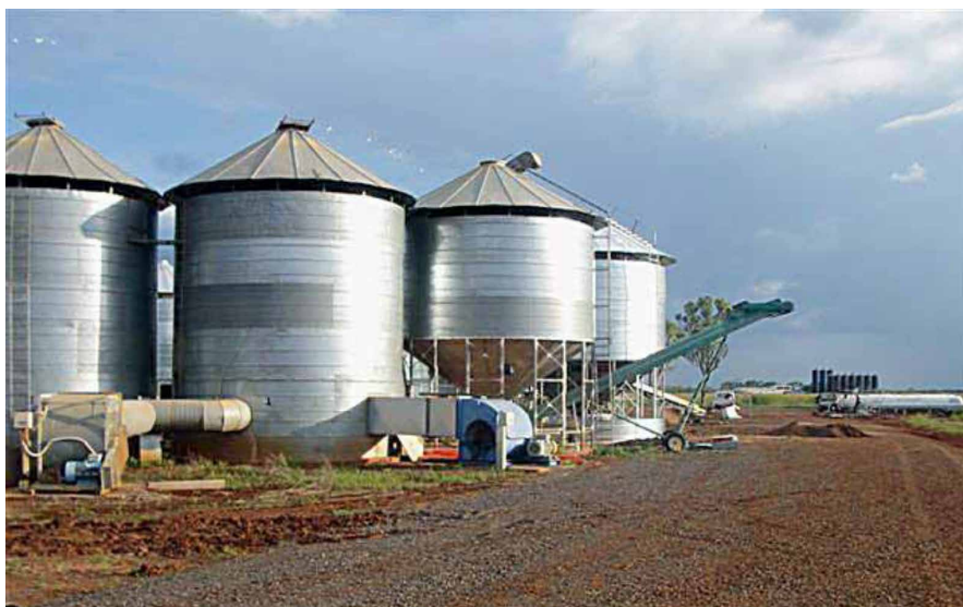
Photo 1: Peanut-drying silos allow pods to dry down to safe moisture content for storage.
