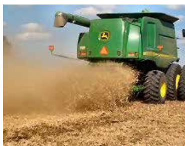
Figure 13: The effluent chaff and the straw need to be spread as wide as the gathering front to facilitate subsequent field operations and eliminate header trails. Bunched material post harvest may interfere with the seeding operation of the following crop. (Photo: AustralianOilseeds Federation)
