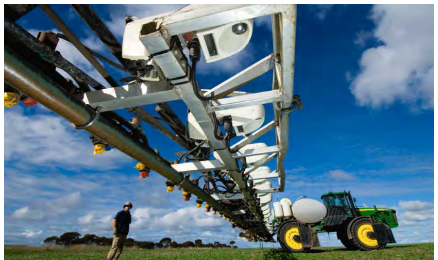
Photo 3: Small sensors on a boom spray will detect broad leaf weeds and a single spray will operate. Precision spraying results in significant savings in herbicides.
