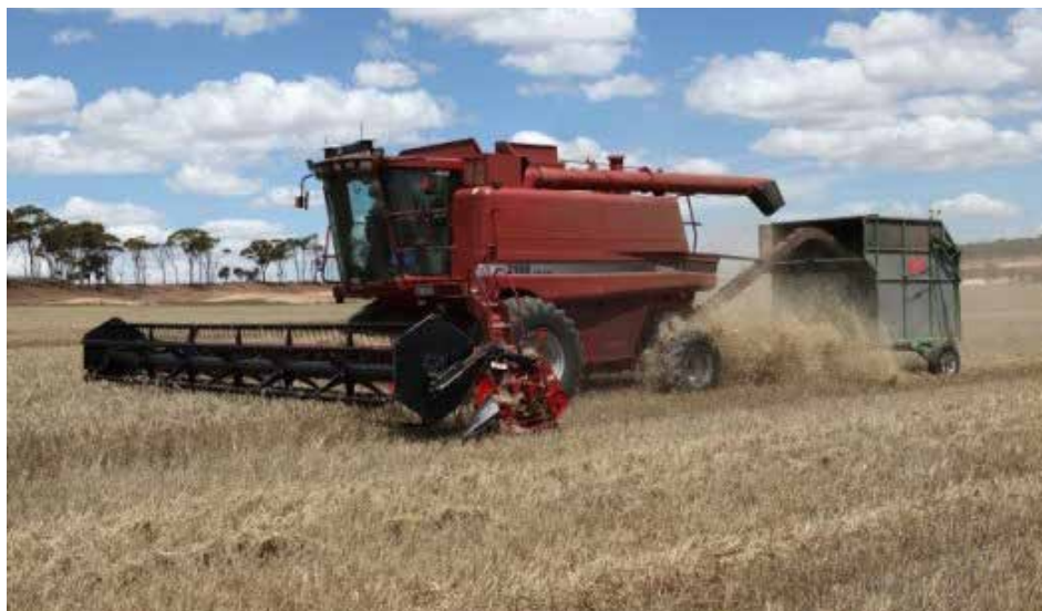
Figure 7: Chaff cart in action at Tarin Rock, WA. (Photo: A. Storrie)
