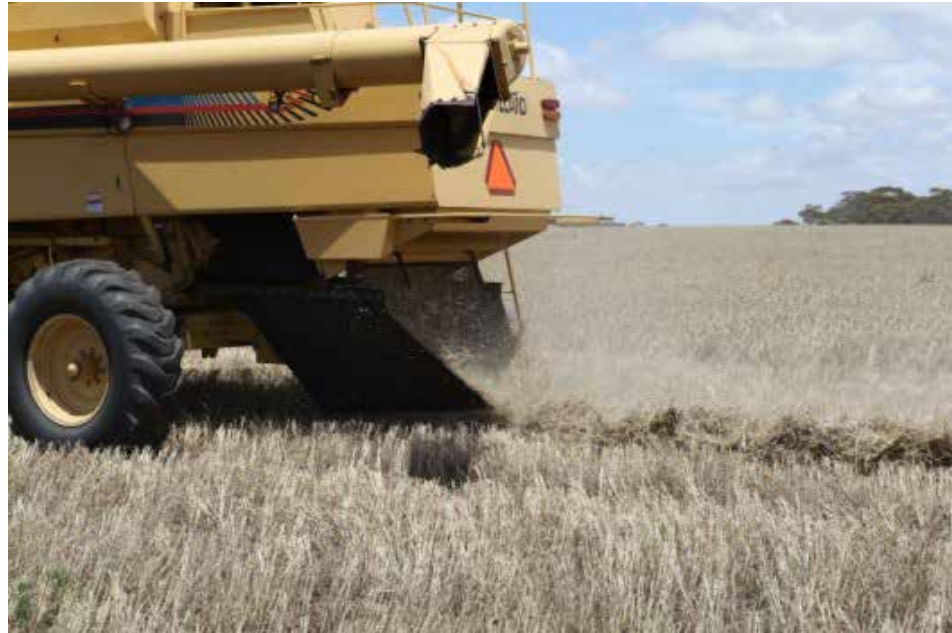
Figure 5: Harvest in action—producing narrow chaff rows for burning in the following autumn. (Photo: A. Storrie)
