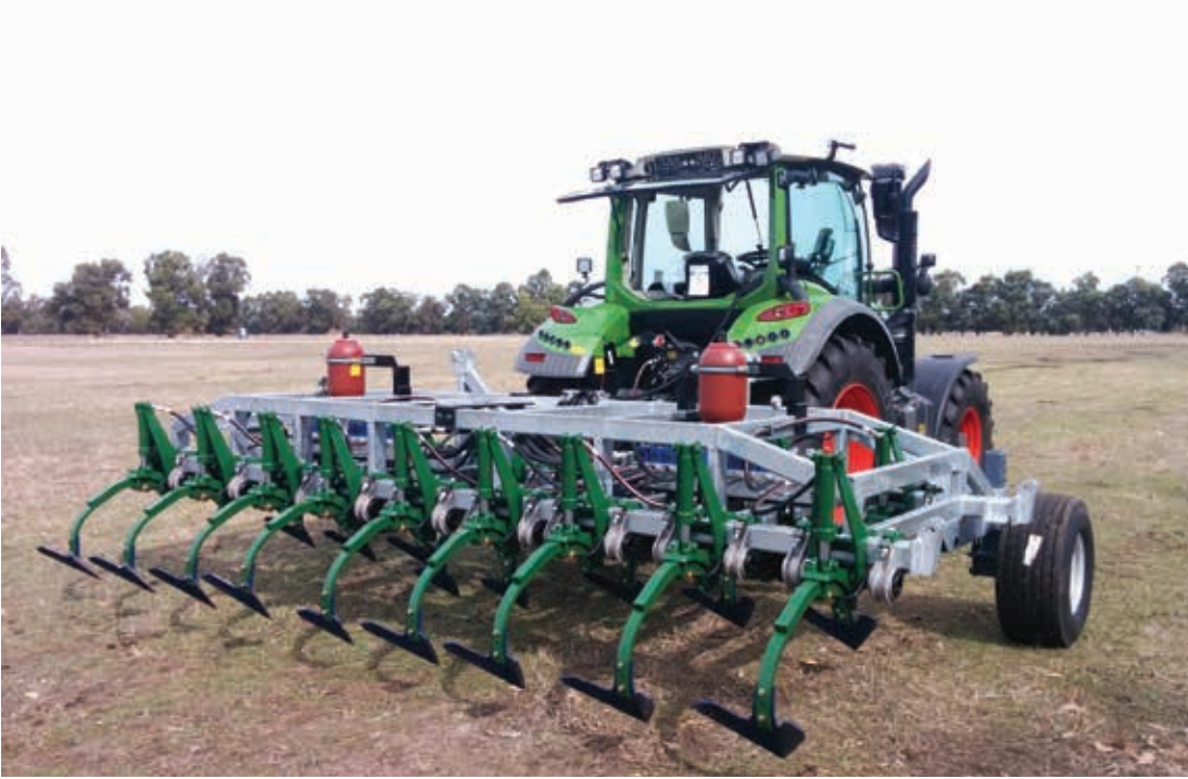
Figure 2. Proof-of-concept rig used in the testing and validation of targeted tillage fallow weed control
