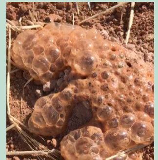
A sample of on-farm lime before (left) and after (right) vinegar is applied. The acid in the vinegar reacts with the carbonate in the on-farm lime to form carbon dioxide gas.
