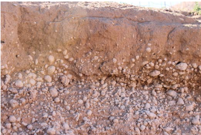
Morrel soil with carbonate nodules near the surface. This source has an NV near 50 per cent.
