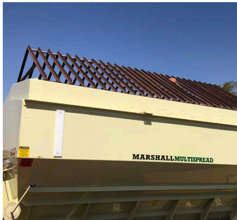
Grizzly screen on spreader takes out large lumps of soil near Bencubbin, WA.
