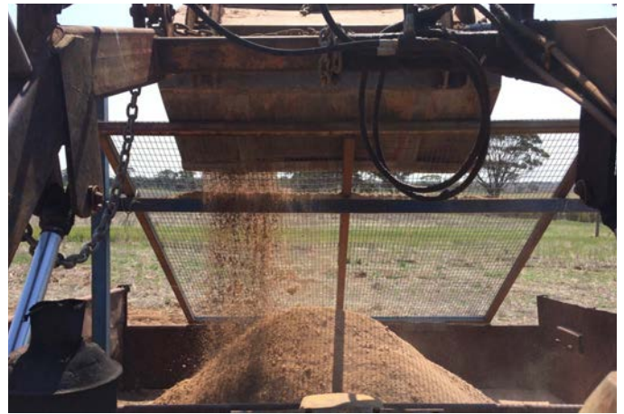
The on-farm lime is screened through 50mm mesh while loading and then taken to the paddock for spreading. PHOTO: MAP IQ
