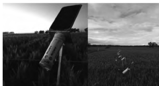
Figure 4. Infrared thermometers (Arducrop) that were used to measure canopy temperatures.
