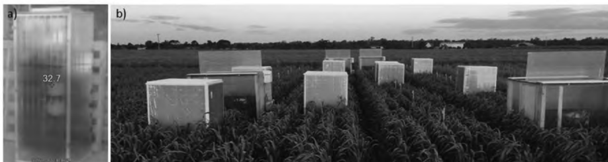
Figure 1. Frost chambers a) Performance testing using visual infrared thermometer, Fluke VT02 (temperature at 32.7°F (0°C)) and b) Simulated frost being applied to wheat to determine impact on yield and ultimately the link between frost induced sterility and proximal sensor response.
