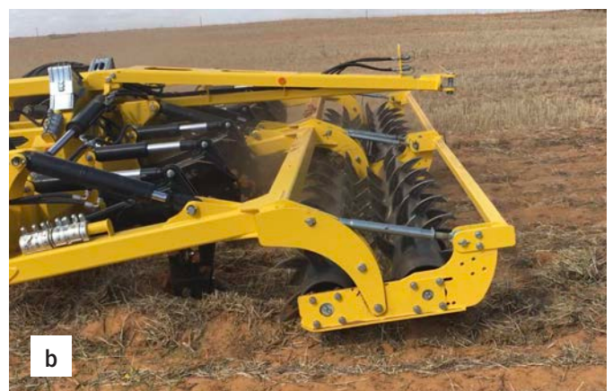
Figure 5: Rollers range from (a) flat steel rollers to (b) rollers mounted on deep ripping machines. Note the reduction in standing stubble following ripping and rolling in Figure 5b.
