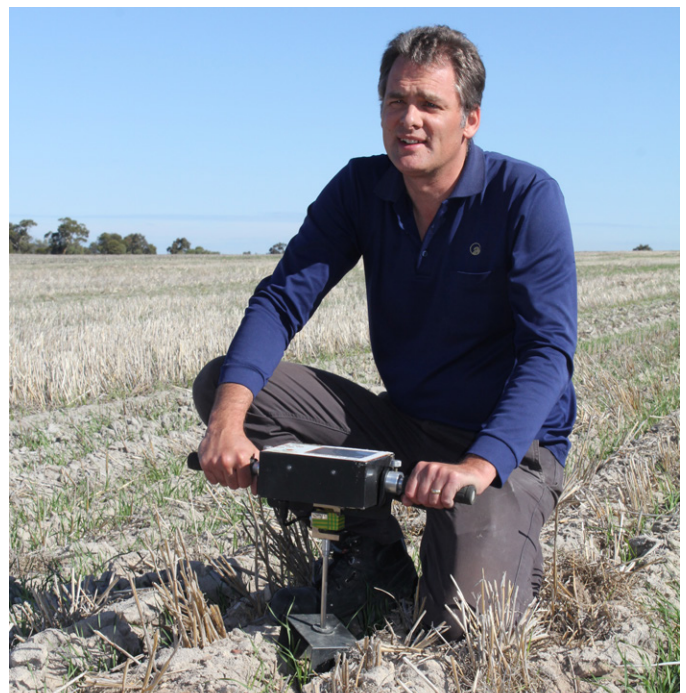
DPIRD WA research officer Dr Stephen Davies tests the soil strength to depth in a deep-ripped plot using a cone penetrometer.
