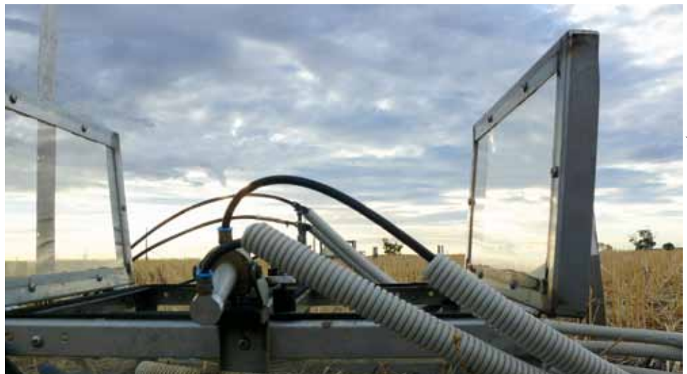
Gas chambers are used to measure greenhouse gas emissions from a soil amended with biochar in Western Australia. Although decreased nitrous oxide emissions have been observed in separate trials in New South Wales, in this trial no difference was recorded between the control and the biochar-amended soil.
