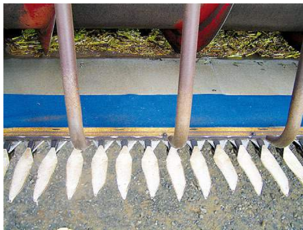
Photo 3: Extension fingers can be fitted to the knife to prevent pods from falling in front of the blade.
