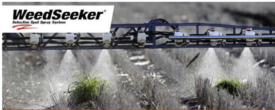
Photo 16: Selective sprayer technology uses optical sensors to turn on spray nozzles only when green weeds are detected.
