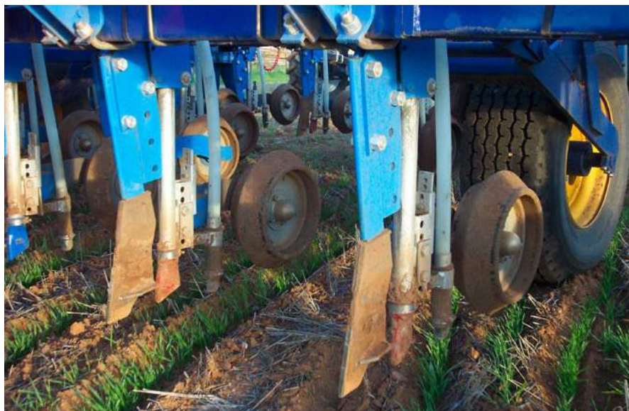
Photo 3: A Primary Precision Seeder fitted with Hydraulic breakout for consistent penetration. It is also fitted are narrow points that form an 'inverted T' slot and is capable of deep or side placement of fertiliser.
