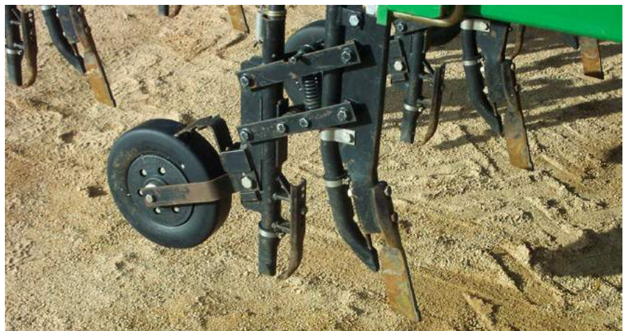
Photo 6: The DBS system parallelogram for uniform seeding depth and deep placement of seed or fertiliser.
