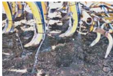
Photo 7: Spray line attached behind each planting tyne/boot dispense inoculants by water injection.
