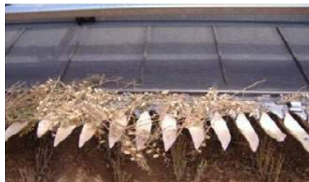
Photo 5: Plastic extension fitted to a draper front.
