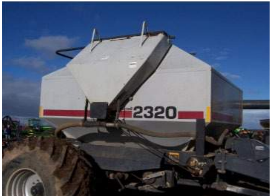
Photo 6: An ‘after-market’ third box fitted to a Flexicoil box to enable application of granular inoculums. Note that granular inoculums cannot be applied mixed with the seed (uneven distribution of seed and/or inoculums occurs). Rhizobia survival is severely jeopardised if granular inoculums are applied mixed with fertiliser.
