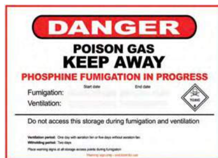
Figure 4: A phosphine warning sign must be clearly displayed.
