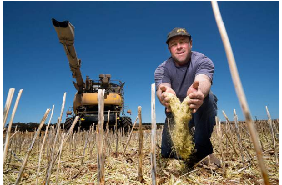
Photo 1: The integrated Harrington Seed Destructor is not a silver bullet but allows growers to destroy weed seed at harvest, facilitating the use of non-chemical weed control as part of an IWM package.
