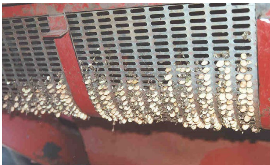
Photo 4: Screen blocked by beans if opening is too large.
