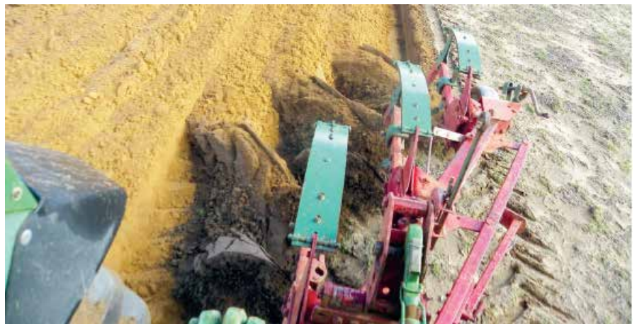
Photo 8: Inversion tillage using a mouldboard plough, as pictured here, has more impact than use of a chisel or disc plough.
