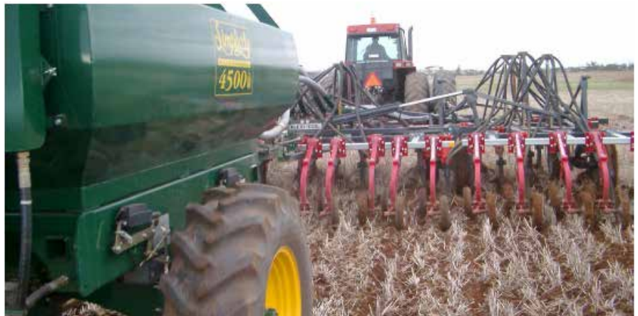
Photo 1: Seeder calibration is important for precise seed placement, and seeders need to be checked regularly during sowing.
