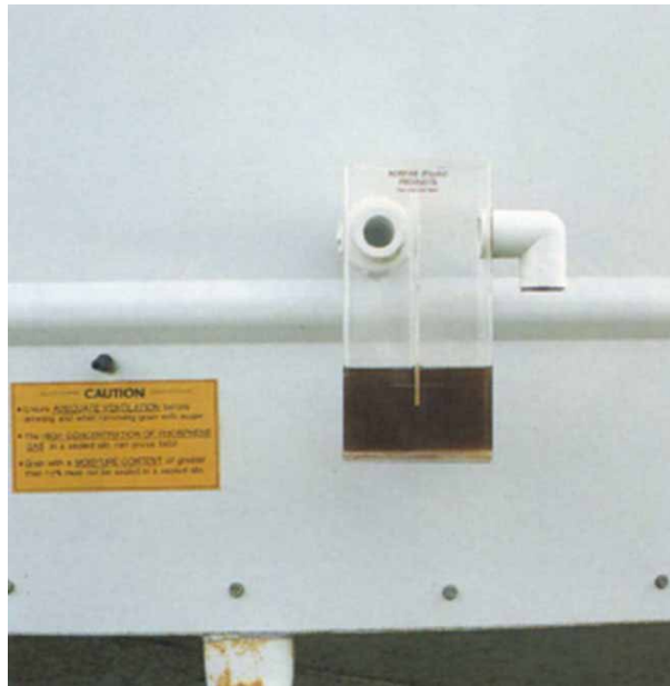
Figure 5: A gas lock on sealed silos gives a quick and reliable means of checking the seal of the silo. Some silos marketed as 'sealed' may not prove to be when tested.
