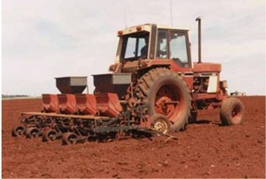
Photo 5: Press-wheels on the planter are essential for good seed–soil contact.
