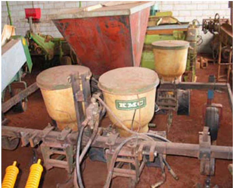
Photo 4: A 4-row planter modified to plant two twin rows.
