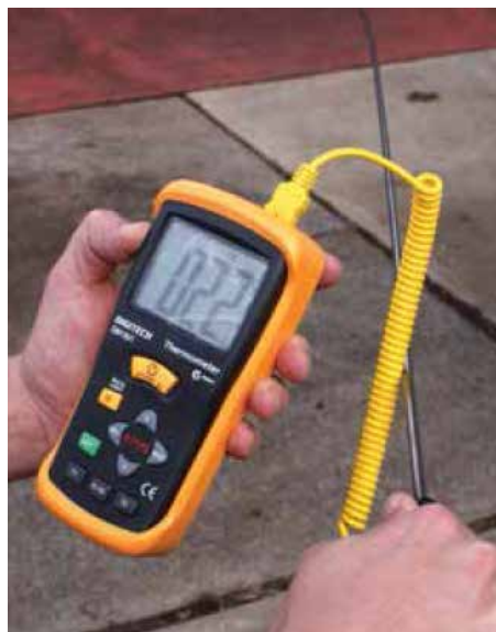
Photo 3: Monitor the effectiveness of the aeration cooling process by checking grain temperature with a temperature probe or a thermometer taped to a rod.
