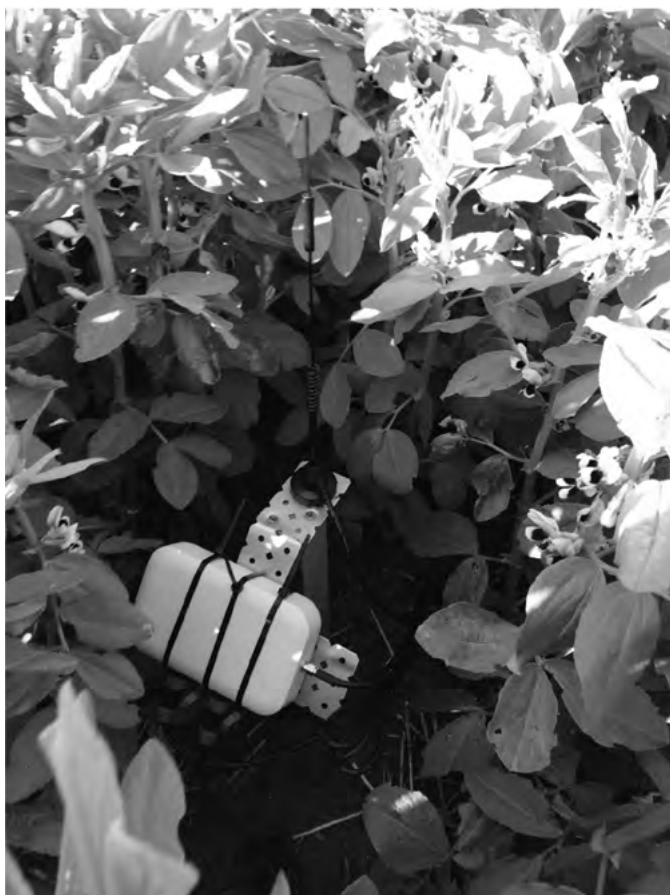
Figure 1. An environmental data logger with telemetry deployed in a faba bean crop.
