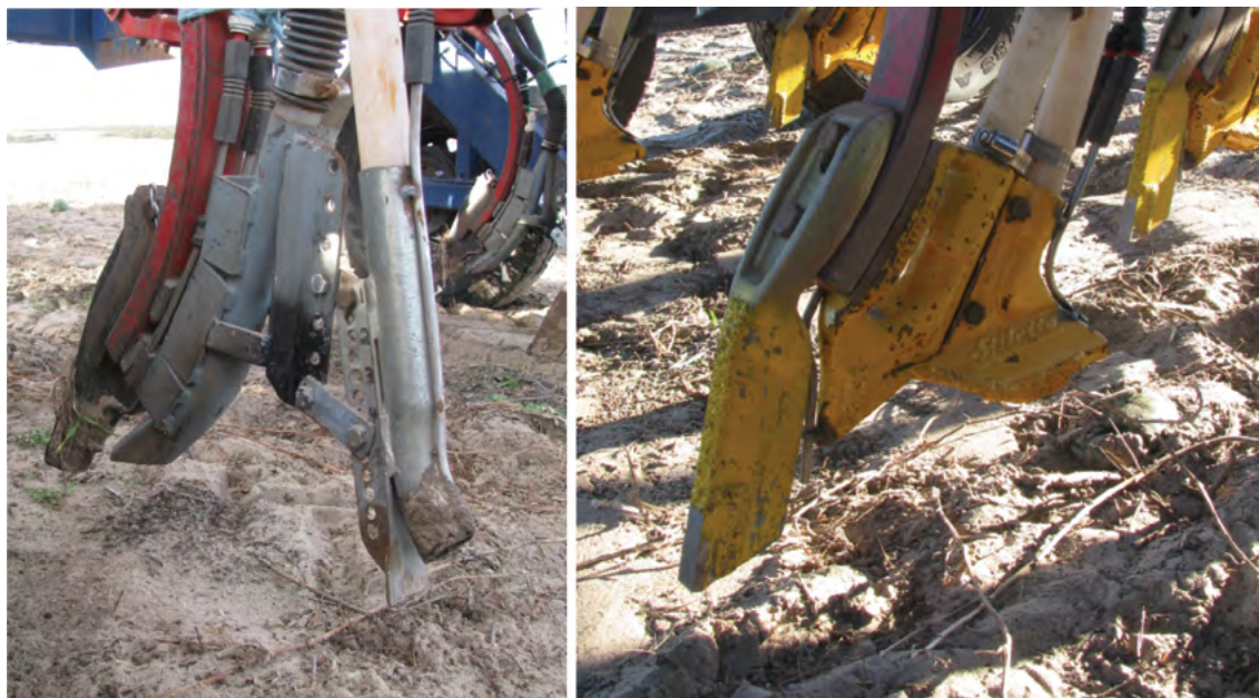
Figure 6. Seeder strategies evaluation trial: Left: Baseline double shoot seeding system used for inter-row and on-row sowing; Right: Side banding double shoot seeding system used for edge-row sowing.
