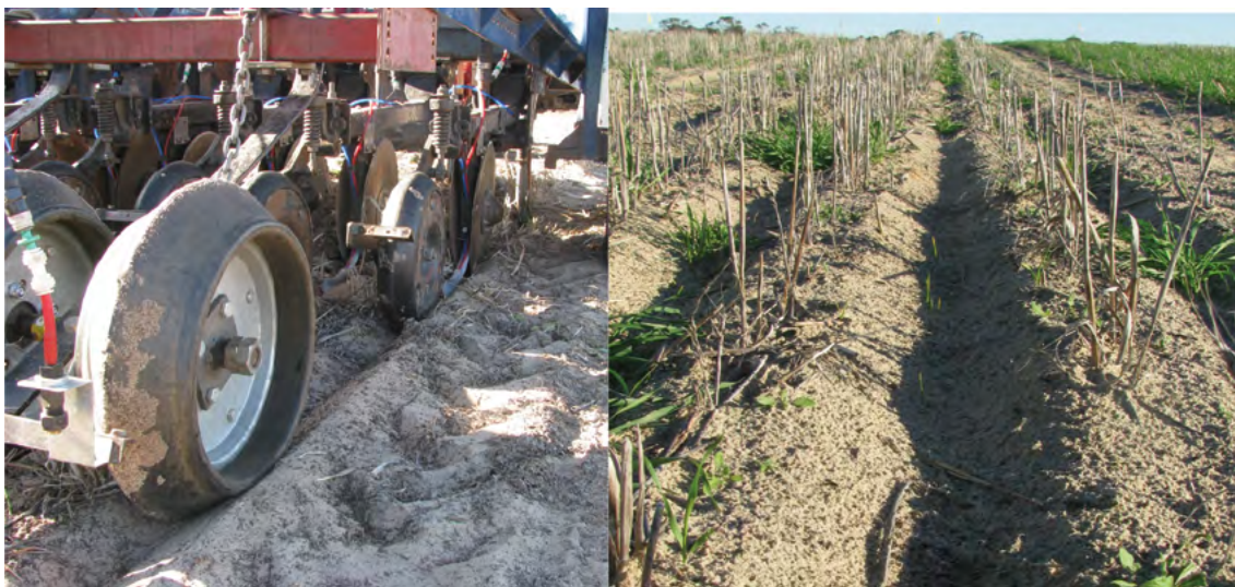
Figure 4. Left: Precision tine-disc seeding system used in the soil wetter evaluation trial; Right: Stable water-harvesting furrows still apparent at 54 days after sowing during 2019.
