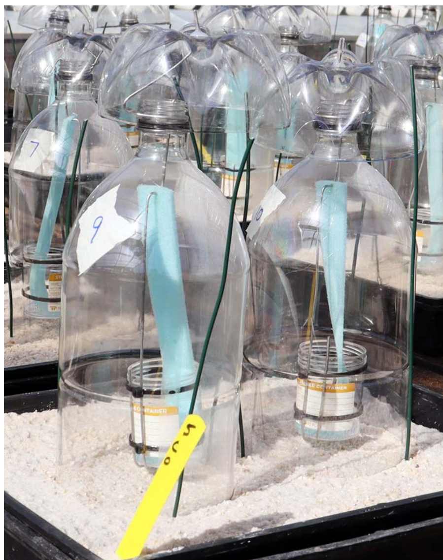
Semi-open passive chambers for measuring ammonia volatilisation losses from soil in the glasshouse.
