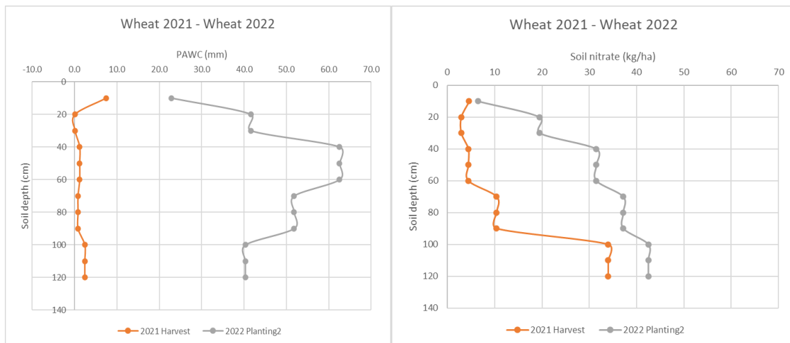
Figure 8. Mean PAWC and soil nitrates at wheat harvest 2021 and wheat planting in 2022. Profile measurements are taken at 0-10, 10-30, 30-60, 60-90 and 90-120cm increments.
