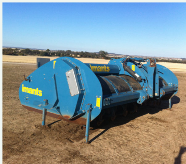
Kym and Fleur Wilkinson have treated 300ha this year with a new Imants 57SX spading machine to help address soil constraints. PHOTO: Kym Wilkinson
