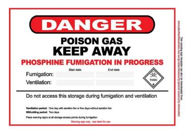
**Figure 3:** A phosphine warning sign must be clearly displayed. They can be downloaded from <u>http://storedgrain.com.au/phosphine-warning-sign/</u>.
