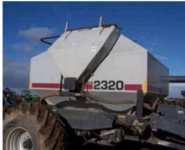
Figure 2: An ‘after-market’ third box fitted to a Flexicoil box to enable application of granular inoculants. Note that granular inoculants cannot be applied mixed with the seed (uneven distribution of seed and/or inoculants occurs). Rhizobial survival is severely jeopardised if granular inoculants are applied mixed with fertiliser.
