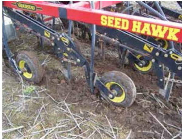
Figure 20: One of several seeding mechanisms for uniform sowing depth using the press wheel for depth control.
