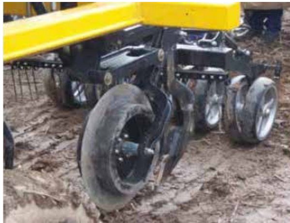
Figure 23: Bio Blade or Cross slot™ disc opener with opening disc and seeding tine, followed by paired press wheels. Note that the seed and fertiliser tube has sharp bends and may not be wide enough to avoid blockages when larger seeded pulses like faba or broad beans are being sown.
