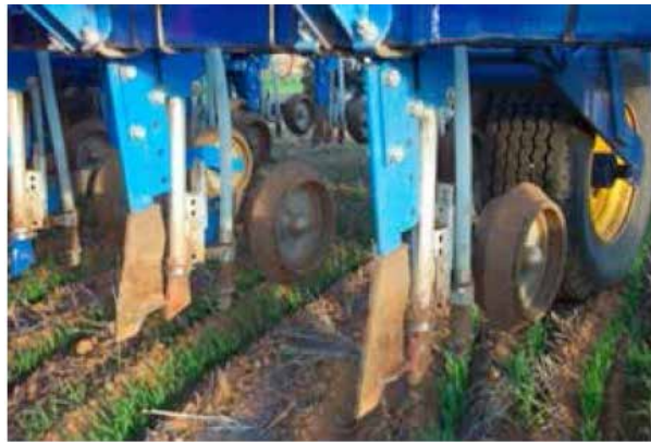
Figure 21: A Primary Precision Seeder fitted with hydraulic breakout for consistent penetration. It is also fitted with narrow points that form an ‘inverted T’ slot and is capable of deep or side placement of fertiliser.
