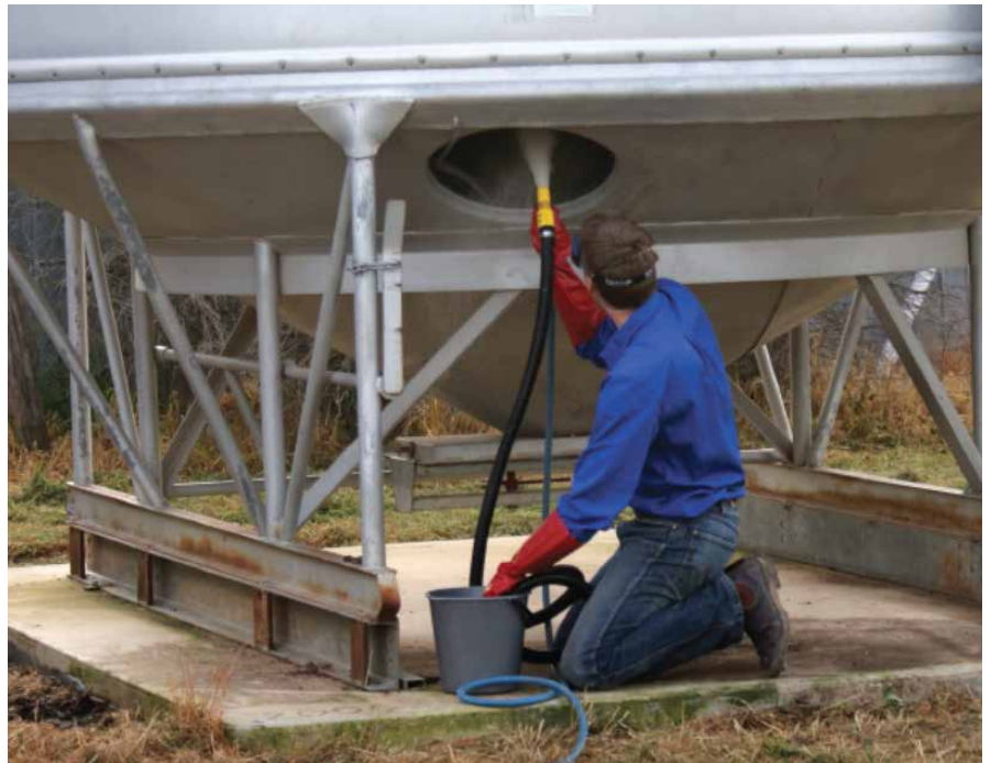
Figure 13: A blower/vacuum or Venturi gun are the best applicators for inert dusts. Aim for an event coat of diatomaceous earth across the roof, walls and base.
