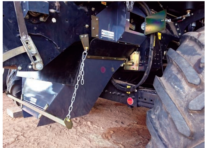
FIGURE 25 New Holland chaff line chute – Westoz Boilermaking.
