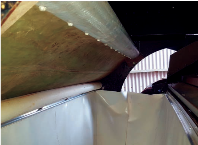
FIGURE 13 Separator baffle inside a Case 7230 fitted with a Mav chopper. Designed by farmer Leigh Bryan to work with his 'Tarpliner' chaff lining chute made from PVC tarpaulin.
