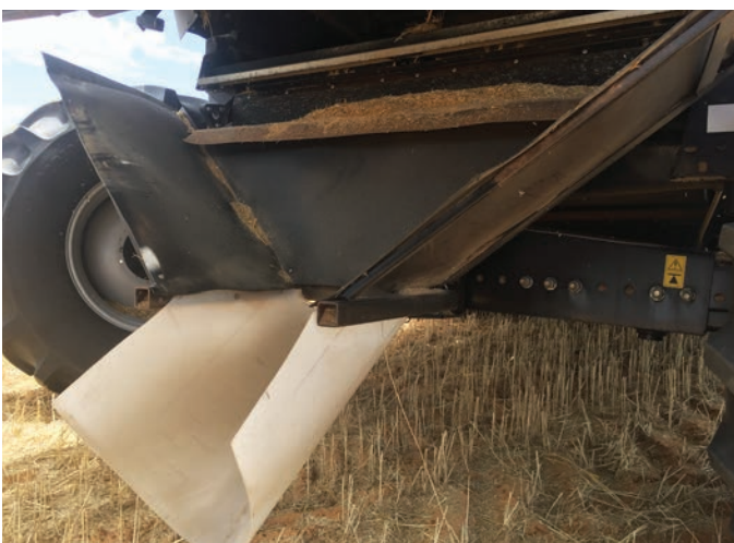
FIGURE 34 Craig Thompson's chaff line chute fitted to a Case 7230. This design works with most 7200, 8200 and 9200 models.
