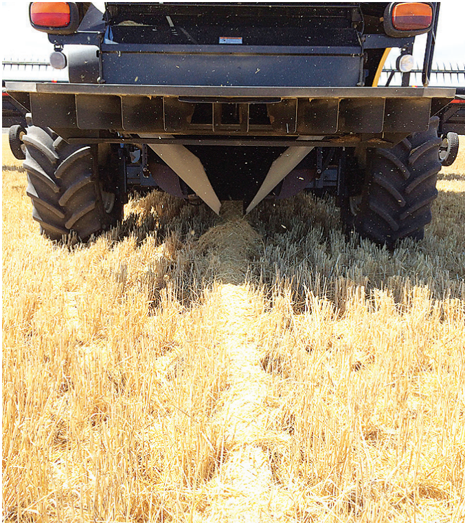
FIGURE 41 The Mic Fels-designed New Holland chaff line chute in action.
