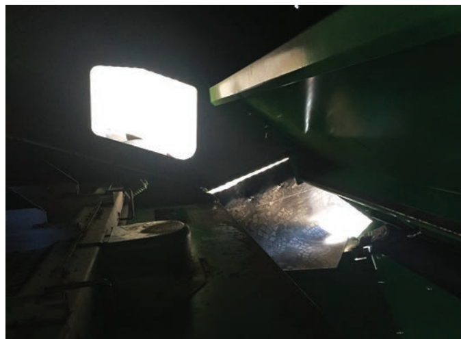
FIGURE 10 Separator baffle inside a John Deere harvester leading into a chaff line chute made by Westoz Boilermaking.
