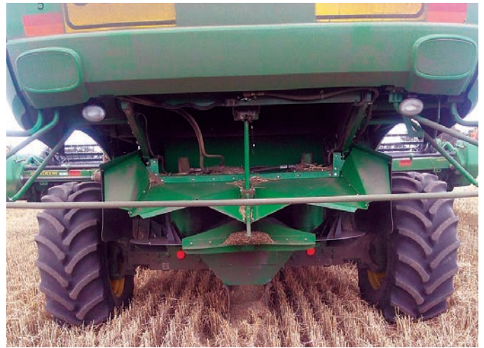
FIGURE 33 The Kohlhagens' chaff line chute in action on a John Deere S670. The straw spreaders are in the normal 'down' position.
