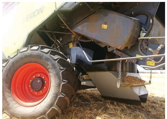
FIGURE 27 Claas Lexion chaff line chute – Westoz Boilermaking.
