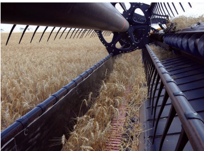
FIGURE 3 Coreflute attached to the finger tyne reel to sweep crop and weed seed heads into the harvester front. This is particularly useful in low-yielding crops (1 t/ha or less).
