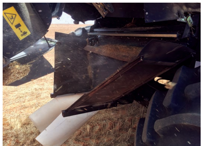
FIGURE 35 Another view of Craig Thompson's chaff line chute with straw spreaders in the 'up' position. The straw spreader cover closes hard against the chaff line chute to make the back of the chute.
