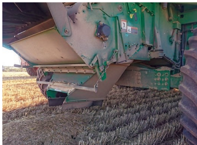
FIGURE 21 STS John Deere chaff line chute – Westoz Boilermaking. A wedge has been inserted at the front of the chopper so it can move it back a little.
