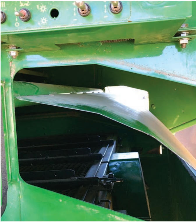
FIGURE 32 The Kohlhagens' chaff line chute on a John Deere S670. This photo shows how the tray behind the sieve was removed to create some room between the sieve and the straw spreaders. The baffle is curved with a rounded leading edge, and a new cover has been made for the sieve controlling mechanism.
