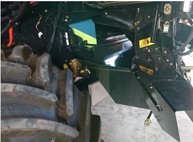
FIGURE 24 Case harvester chute – Westoz Boilermaking. The straw spreaders close down on the back of the chute. The spreader is fitted with a cover to minimise weed seeds being sucked in.
