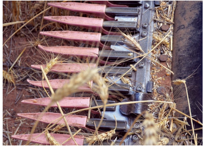
FIGURE 2 Primary sales knife extensions used to improve crop and weed seed capture.
