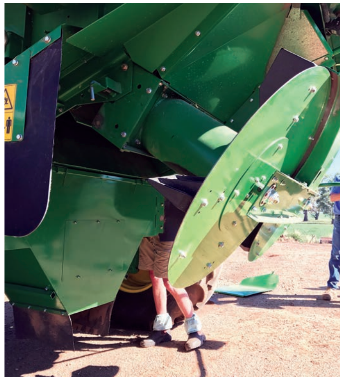
FIGURE 31 The Kohlhagens' chaff line chute on a John Deere S670. The straw spreaders are in the 'up' position for the photo, but while harvesting they operate in the normal 'down' position.
