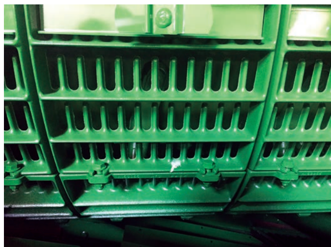
FIGURE 7 The rear grates of John Deere harvesters are more 'closed up' than other makes of harvester.
