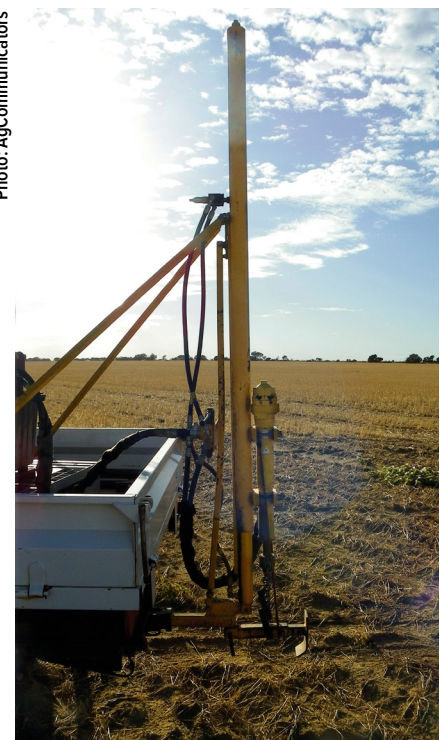
Deep core samples are taken using a ute-mounted hydraulic ram probe.
