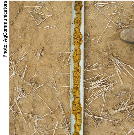
Deep core sample taken using hydraulic ram probe.
