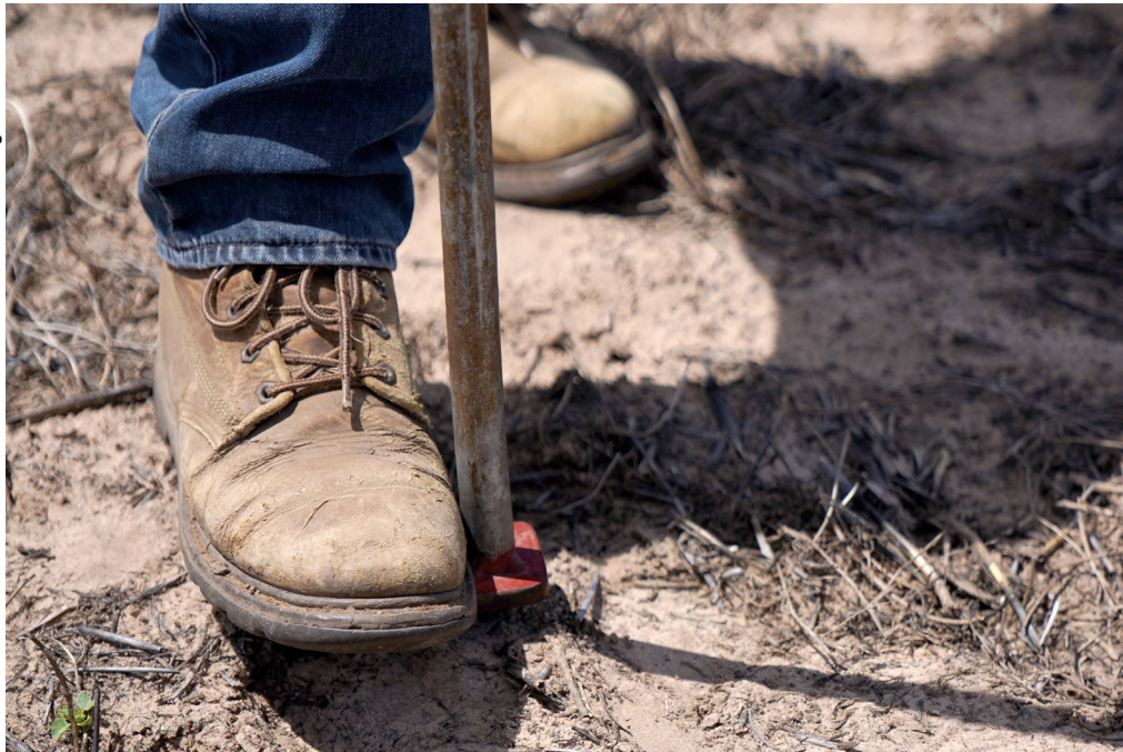
Topsoil samples are taken from the top 10cm of the soil surface using a pogo stick sampler.
