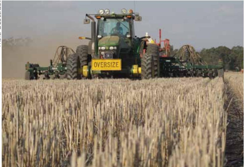
*A gradual low-cost approach to machinery changeover was taken in this 9-metre system at Wagga Wagga, NSW. A Horwood Bagshaw seeder width was matched to the existing header, then axles on boom and spreader converted to 3m in the farm workshop. JD front wheel assist tractor on 3m is used for all operations. A new disc seeder was purchased in 2013 to complement the no-till continuous cropping and stubble retention system.*
