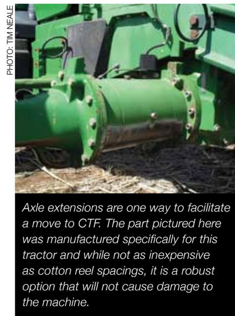
*Axle extensions are one way to facilitate a move to CTF. The part pictured here was manufactured specifically for this tractor and while not as inexpensive as cotton reel spacings, it is a robust option that will not cause damage to the machine.*
