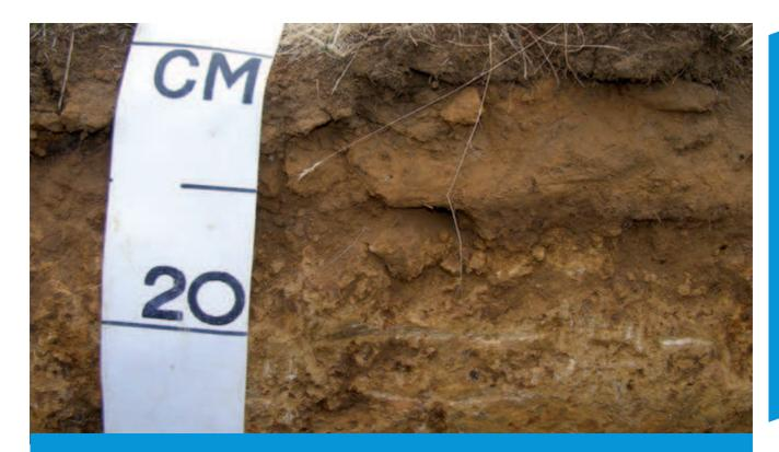
**Plate 5.1** A sub-surface compaction layer shows a dense impenetrable soil layer. *Source: Tim Overheu, DAFWA*
