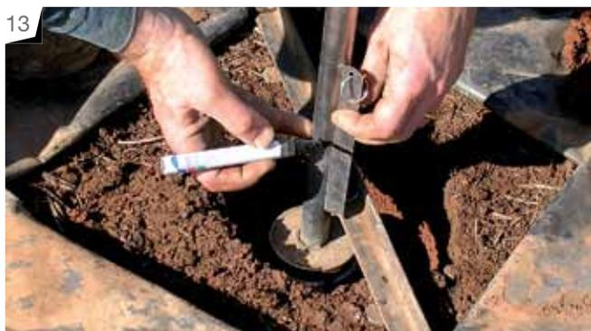
Photo 13: Referencing sampling depth. The sampler is placed in the hole and the depth of the core sample measured and marked on the shaft of the sampler using the datum pins as reference. The corer is driven into the soil until the mark reaches the line of the datum pins. Driving the sampler past the reference line will result in compaction of the sample within the corer head.
