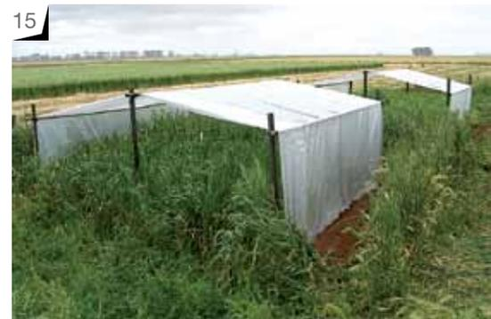
Photo 15: Rain-exclusion tent in place. Duct tape on the pipes prevents chaffing. The plastic cover lies between the posts to simplify the attachment of the tubes. At the minimum 20° pitch, the cover must be tight to shed water.
