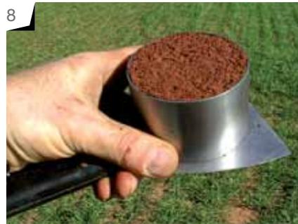
Photo 8: A BD sample ready for bagging. Note the use of a paint scraper to hold the coring ring whilst trimming the sample. Two such scrapers are useful when turning the sample over to trim.
