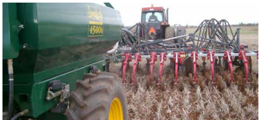
Photo 1: Seeder calibration is important for precise seed placement and seeders need to be checked regularly during sowing.
