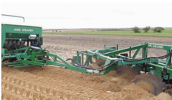
Figure 3.46: John Shearer high-work-rate prototype full inversion disc plough and one-pass seeder.
