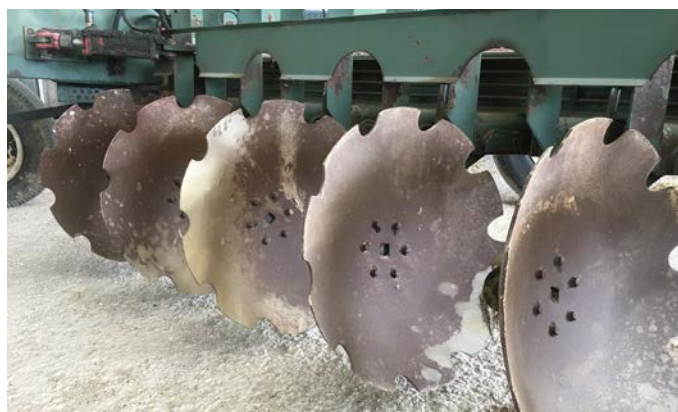
Figure 3.7: John Shearer one-way 5GP plough, modified to fit Plozza discs.
