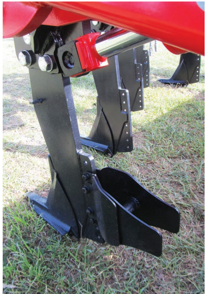
Figure 3.33: Commercial inclusion plates exist in many shapes and sizes, and evaluation using computer simulation can help guide their selection and settings for best results in the paddock.
