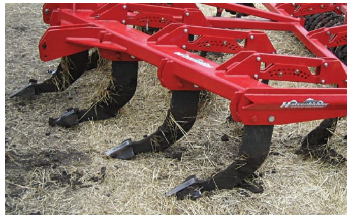
Figure 3.14: Parabolic narrow shank ripper fitted with winged high lift points for maximum soil loosening depth capacity.
