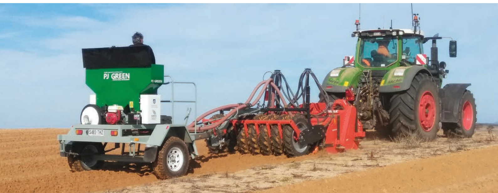
Figure 3.17: Research in the southern region over the past seven years has highlighted consistent crop benefits from 'mixing by spading' in a variety of deep sand and surface amendment contexts.
