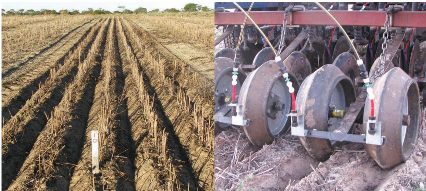
Figure 2.7: Water-harvesting stable furrows (left) shaped by wide V-shouldered press-wheel tyres (right) help soil wetter effectiveness, while maintaining standing stubble is often best practice for minimising furrow infill over time.
