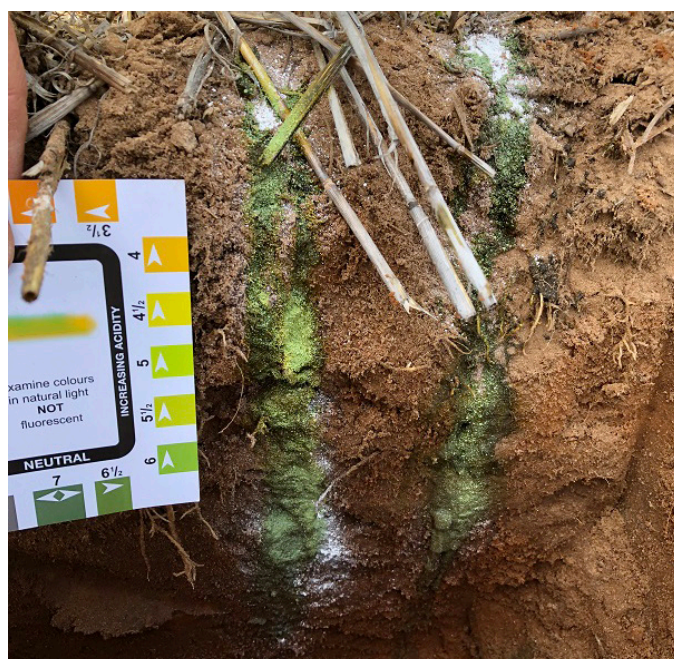
Figure 1.2: Paddock pH indicator testing. The ideal range is between 6.5 and 7.5. Acid layers will show as bright green or yellow colours. Alkaline layers will be deep purple.
