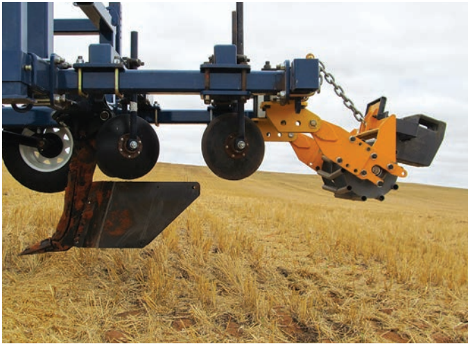
Figure 3.34: Proof-of-concept active inclusion system (top) is able to maximise inclusion capacity (bottom-left) and achieve a consolidated and levelled seeder-ready finish (bottom-right).
