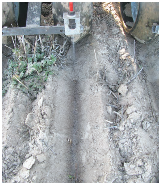
Figure 2.8: Application of soil wetter behind water-harvesting 'open V' press-wheels via a narrow (15 degree) flat fan nozzle achieving a stable 3cm wide spray footprint at the base of a firm furrow.
