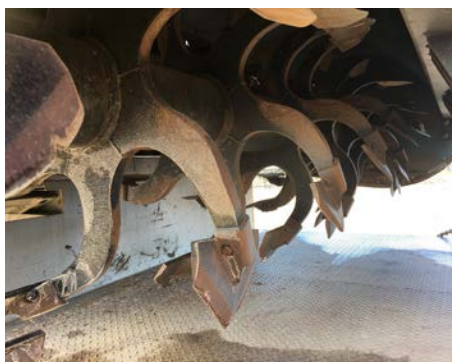
Figure 3.4: Triangular-shaped spades on curved tynes are fixed to a central shaft that rotates at \sim 90\text{revs/min}^{10} .
