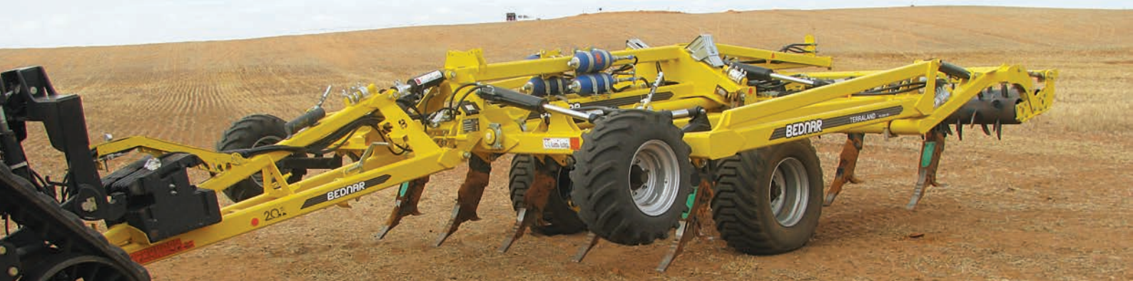
Figure 3.9: High-disturbance ripper using narrow-spaced delving tynes to bring up soil from deeper layers, combined with levelling spike rollers to provide a levelled finish.
