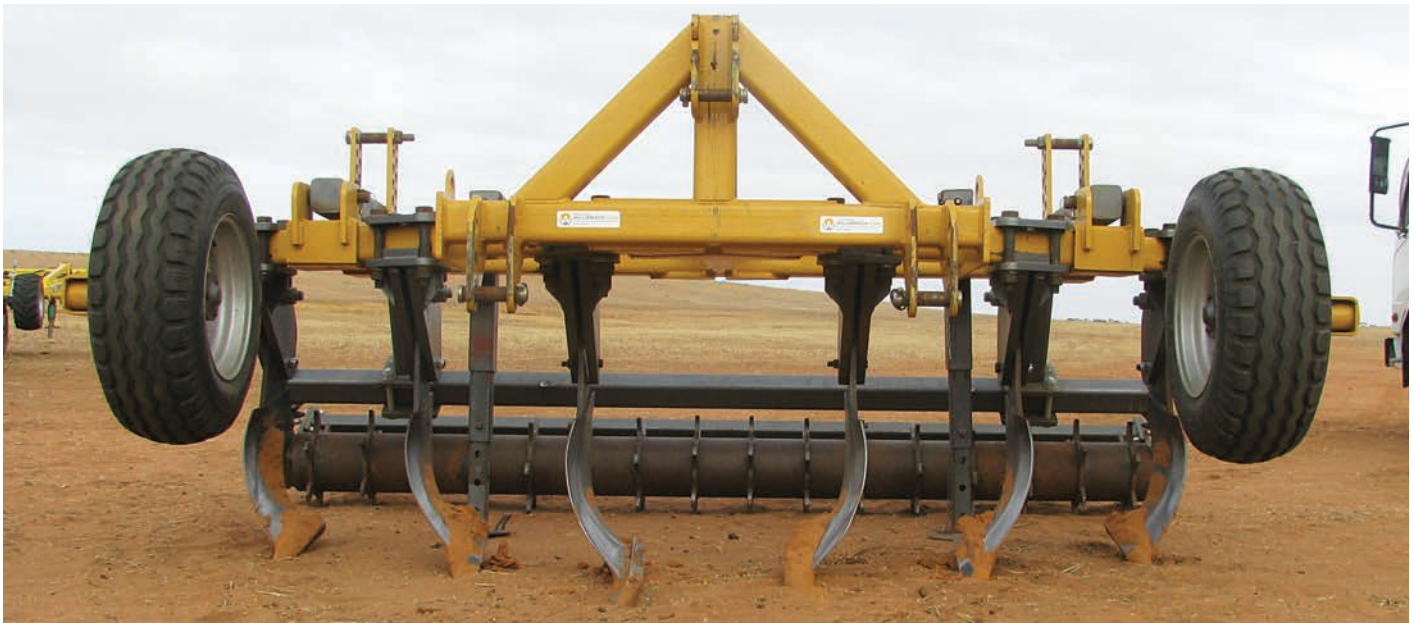
Figure 3.15: Curved slanted narrow shank ripper for low-disturbance loosening.
