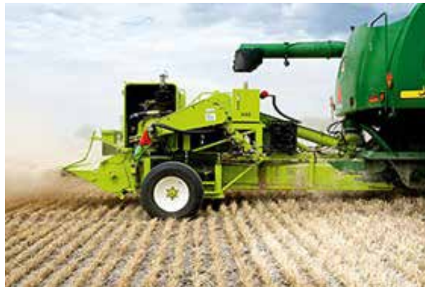
Photo 16: Harrington Seed Destructor at work in the paddock.
