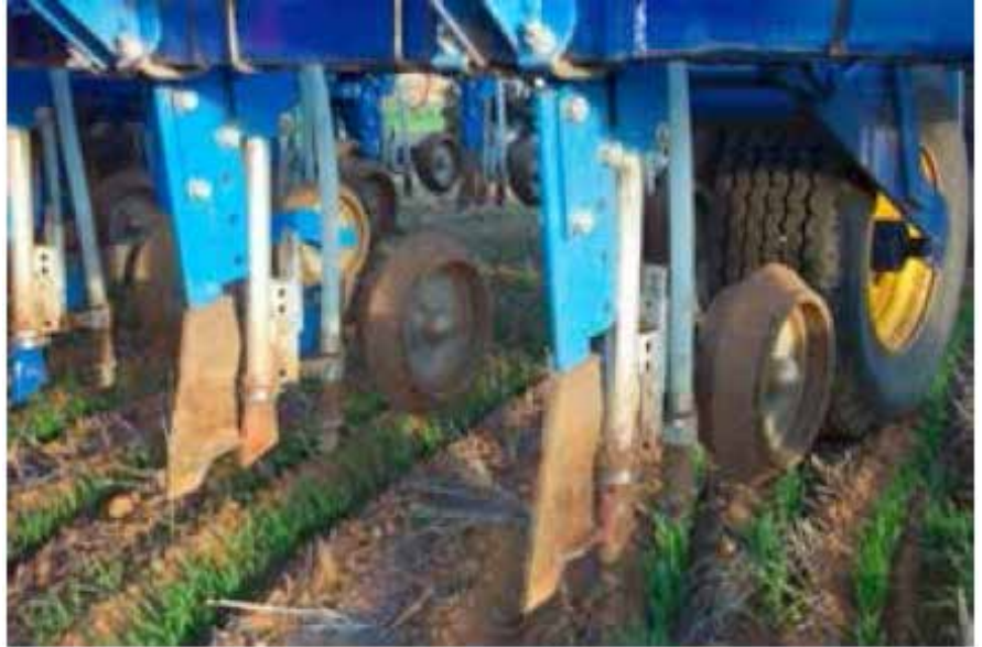
Photo 13: A Primary Precision Seeder fitted with hydraulic breakout for consistent penetration. It is also fitted with narrow points that form an 'inverted T' slot and is capable of deep or side placement of fertiliser.
