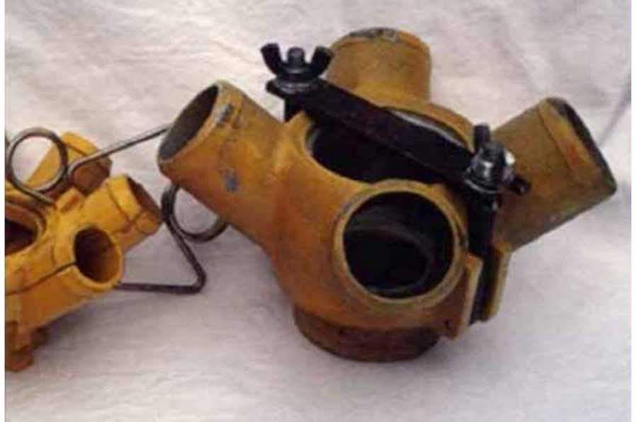
Photo 11: Conversion heads, such as this one for a Connor-Shea airseeder, allow large seeds such as broad beans, faba beans, and Kabuli chickpeas to be sown with ease.
