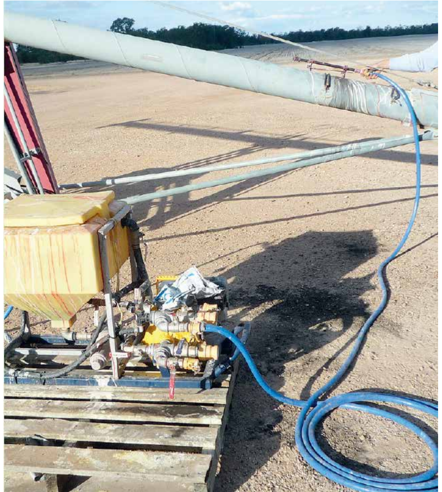
Photo 3: Pumping a slurry of rhizobia inoculant into the auger to coat seed before sowing.
