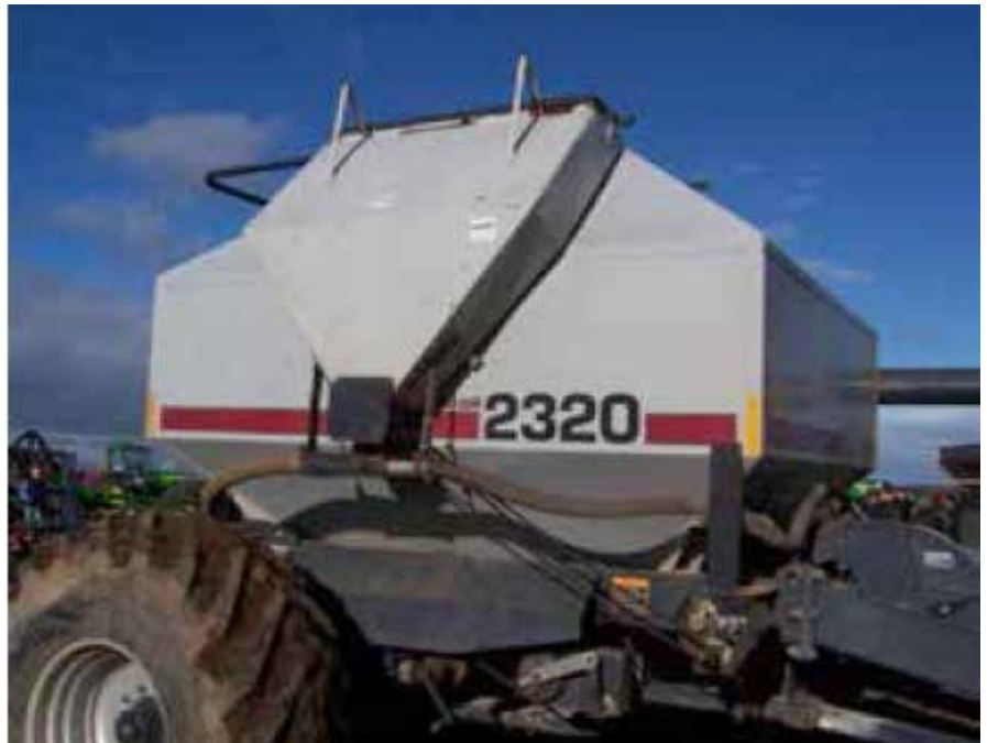
Photo 2: An ‘after-market’ third box fitted to a Flexicoil box to enable application of granular inoculums. Note that granular inoculums cannot be applied mixed with the seed (uneven distribution of seed and/or inoculums occurs). Rhizobial survival is severely jeopardised if granular inoculums are applied mixed with fertiliser.
