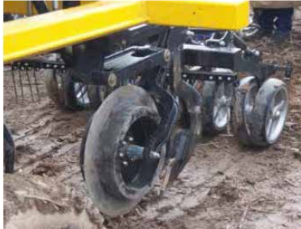
Photo 15: Bio Blade or Cross slot™ disc opener with opening disc and seeding tine, followed by paired press wheels. Note that the seed and fertiliser tube has sharp bends and may not be wide enough to avoid blockages when larger seeded pulses like faba or broad beans are being sown.
