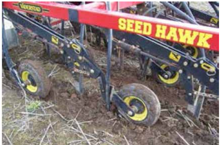
Photo 12: One of several seeding mechanisms for uniform sowing depth using the press wheel for depth control.
