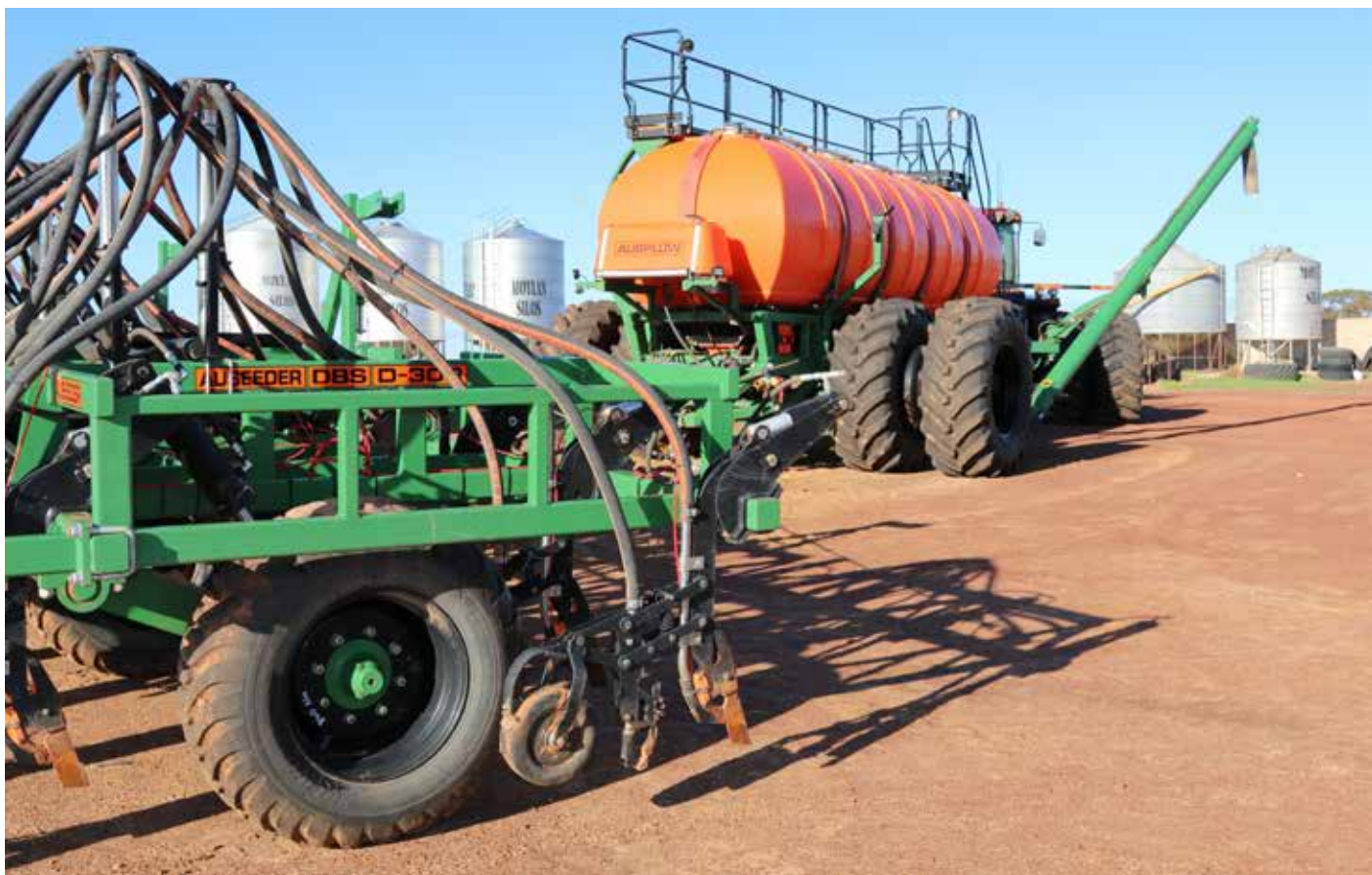
Rather than sowing deeper, the Wilsons will rip as deep as possible beneath the seed with their DBS bar to improve capillary rise and crop rooting depth.
