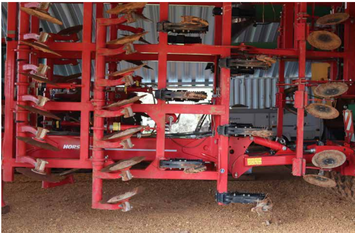
Originally designed to mix in heavy stubbles in Europe, Ben Strickland purchased a Horsch Tiger to mix their lime and corrected pH soils, which are now just in that topsoil, as well as breaking the hard pan and mixing the organic matter.
