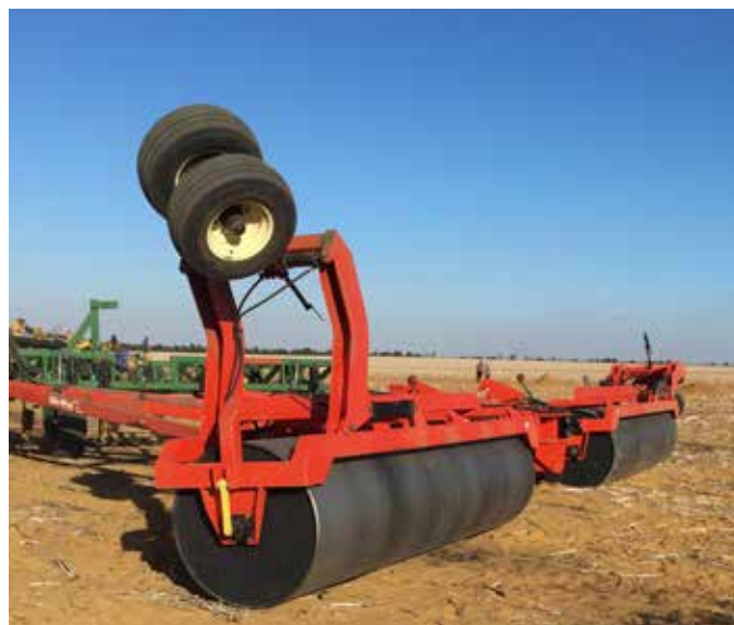
A weighted roller is towed to achieve a firm, even seed bed.
