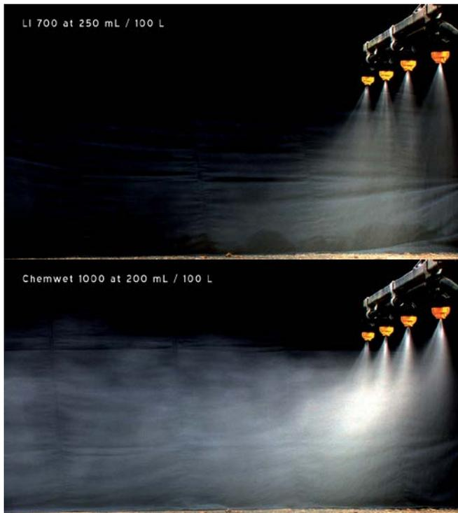
**Figure 1d:** The images above show how two adjuvants with the same nozzle set-up and environmental conditions can result in completely different characteristics of the spray solution. Droplet size is changed causing drift and less product reaching its target. The top image is a spray solution with the surfactant LI-700® at 250 ml/100L while the bottom image is Chem-wett 1000 at 200 ml/100L.
