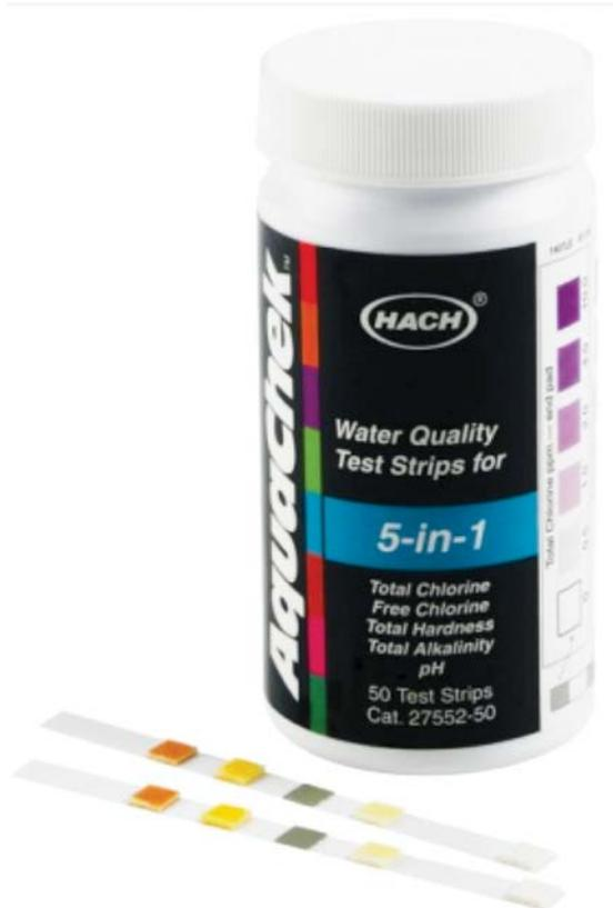
Water quality test strips can be used to assess pH and water hardness in the field.
